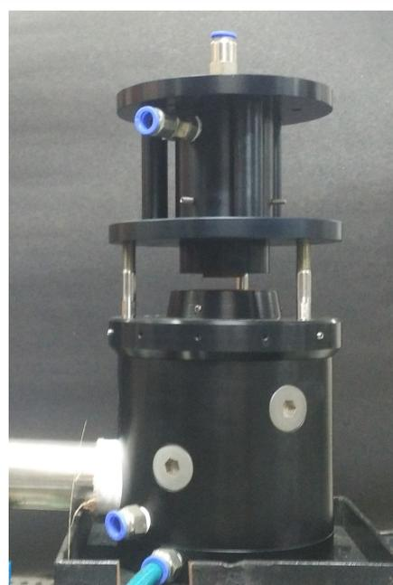
Figure 1: Schematic of the counter-flow burner setup.
